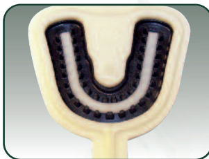
Stampo in gomma e linguetta spaziatrice Rubber box and flap for model casting
